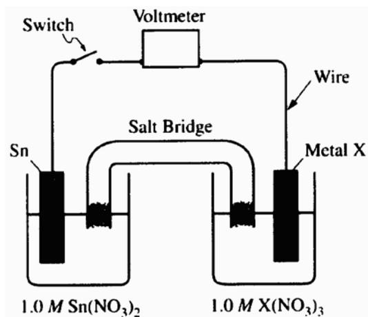
An electrochemical cell is constructed with an open switch, as shown in the diagram above. A strip of Sn and a strip of unknown metal, X are used as electrodes. When the switch is closed, the mass of the Sn electrode increases. The half-reactions are shown below.
