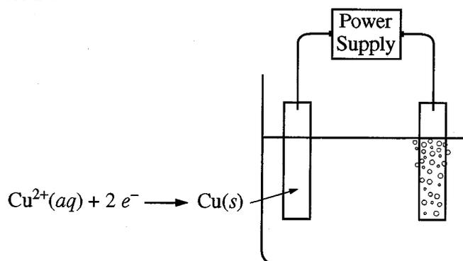
An external direct-current power supply is connected to two platinum electrodes immersed in a beaker containing  $1.0\text{ M CuSO}_4(\text{aq})$  at  $25^\circ\text{C}$ , as shown in the diagram above. As the cell operates, copper metal is deposited onto one electrode and  $\text{O}_2(\text{g})$  is produced at the other electrode. The two reduction half-reactions for the overall reaction that occurs in the cell are shown in the table below.
